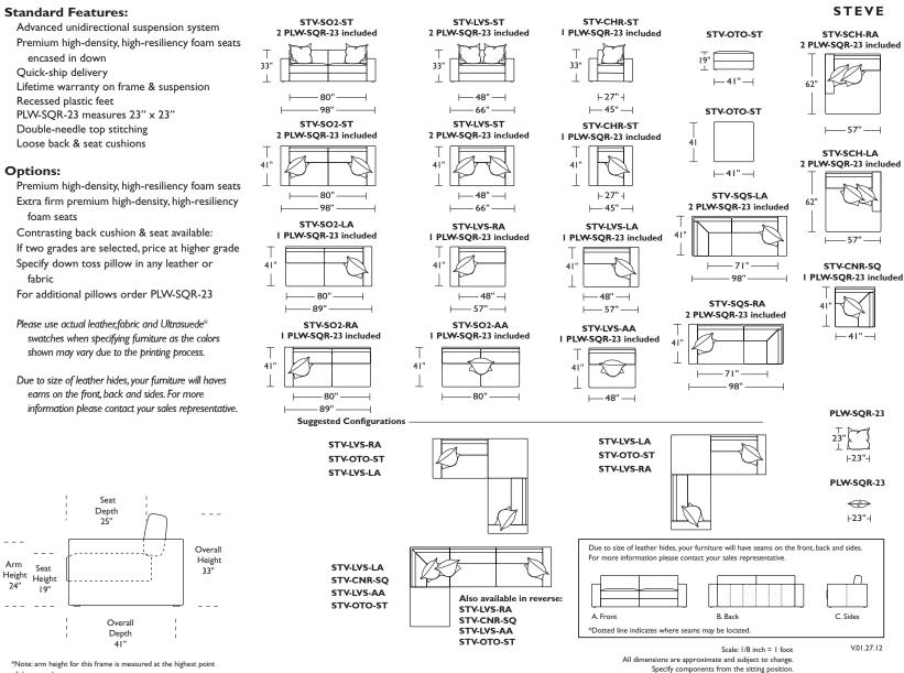
\*Note: arm height for this frame is measured at the highest point of the curved arm.
